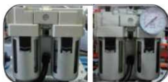
Left type of FRL is standard one Right type of FRL is for option
